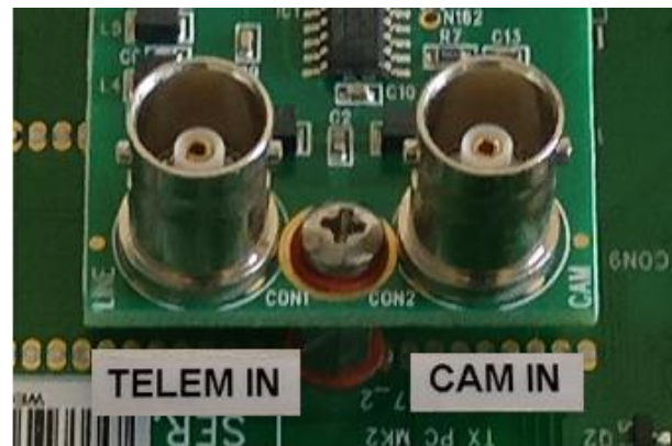
Video Connections controller and camera
