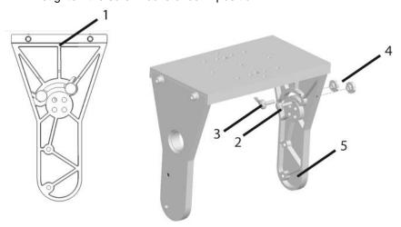
Fig. 8 Over the Top tilt limit adjustment
