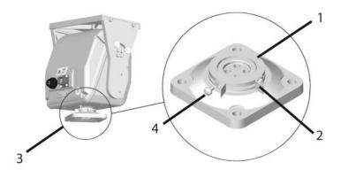
Fig. 7 Setting the Pan end-stops
